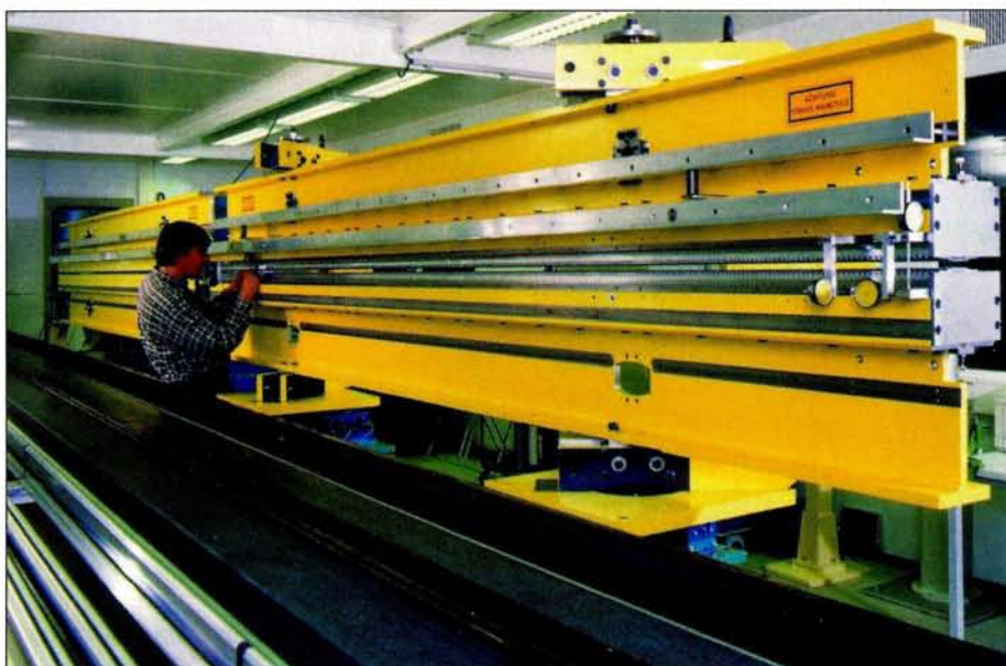
The magnetic “undulator” at the heart of the new free electron laser at DESY has to shake transmitted electron beams with a precision of 20 \mu\text{m} .
